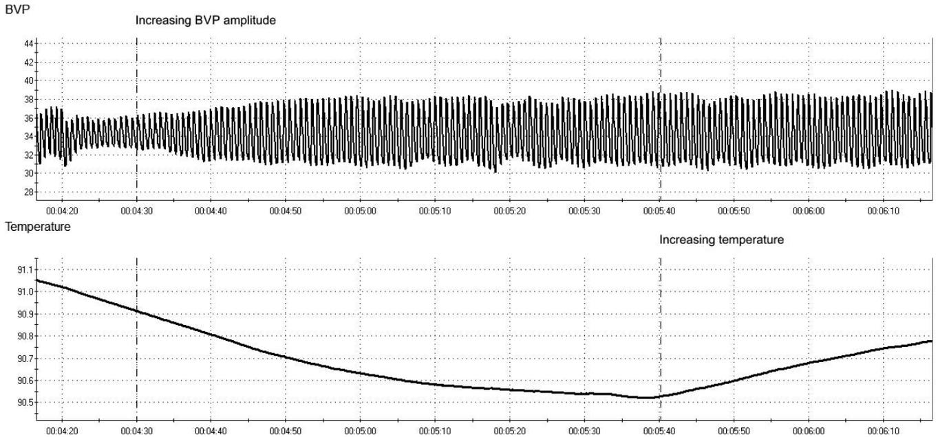
Figure 2. Comparison of photoplethysmograph and thermistor signals.
