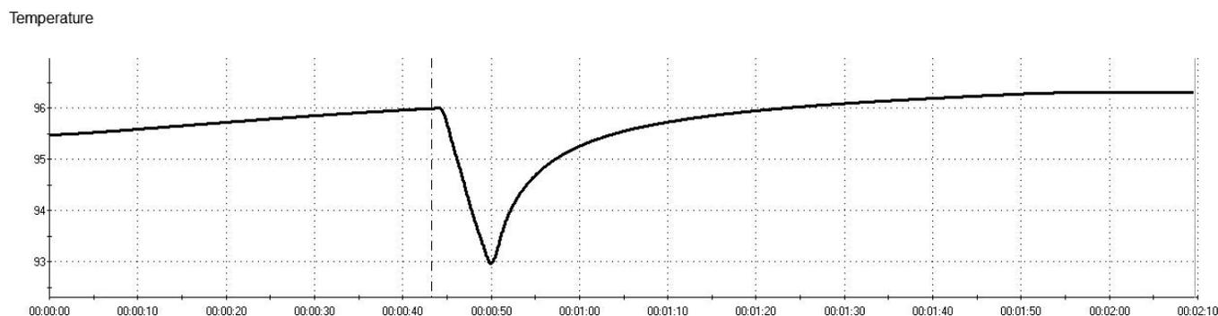
**Figure 7.** Thermistor decoupling due to movement.
